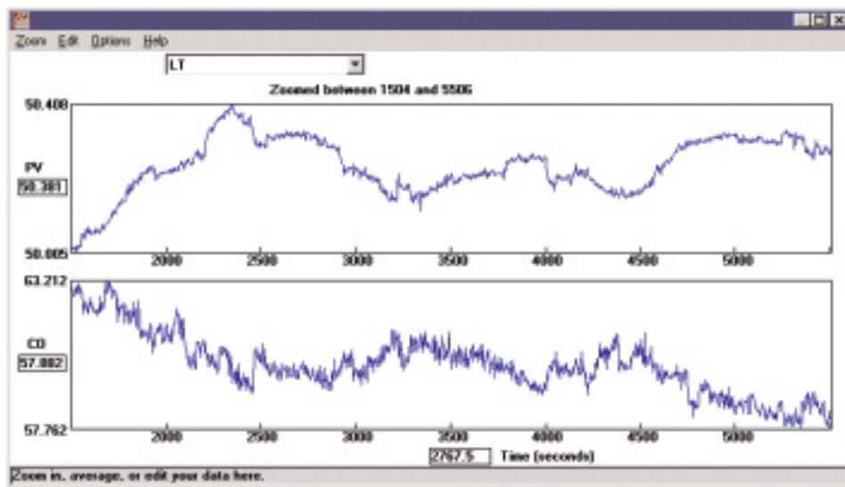
Figure 2. The closed-loop time response for the machine chest level control
